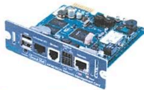
Schneider UPS Network Management Card 2 with environment monitoring, out-of-band access, and modbus
